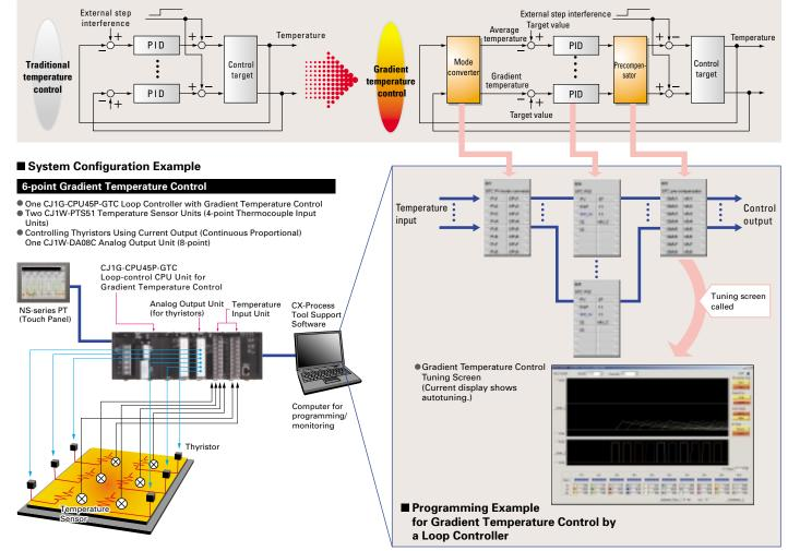
Note: Real programs require gradient SP mode conversion blocks to input settings to each PID block.
