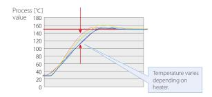
Driving multiple heaters independently cause heating interaction between each area of the metal plate. This means and perfect temperature uniformity is almost impossible.
