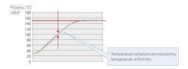
Temperature variations reduced by controlling temperatures based on the set points corrected for each separate heater using the set points and process values.
